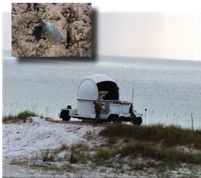
Below, an optical tracking unit with a digital imaging-based kineto tracking mount is hauled on a trailer to a surveyed sites. Inset photo: unexploded ordnance
